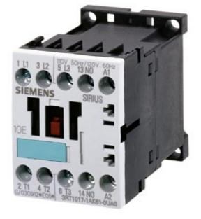
CONTACTOR, AC-3 5.5 KW/400 V, 1 NO, AC 230 V, 50/60 HZ, 3-POLE, SIZE S00, SCREW CONNECTION
