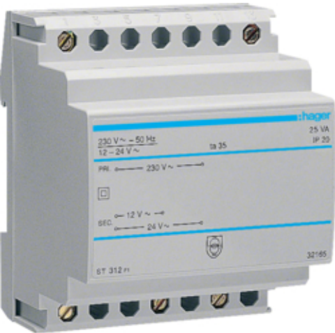
Veiligheidstransformator 25 VA, Usec 12/24 VA, Uprim 230 VAC
