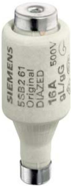
DIAZED FUSE LINK 500V F.CABLE AND LINE PROTECTION OP.CL.GL,SZ.DII,THREAD E27,16A
