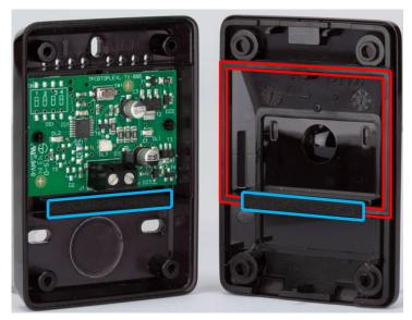
All models are provided with a **co- printed seal** (on the cover) and with a **closed cells seal** on the cable's passage area, thus to always guarantee the maximum protection of the PCB in any weather conditions as well as to avoid the entrance of insects.
