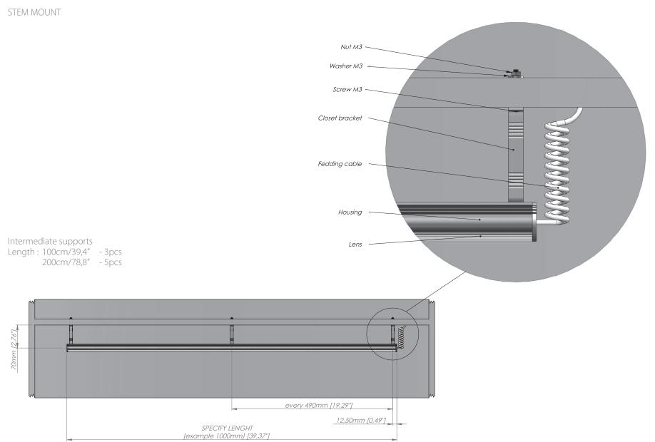
Intermediate support arm for Alu-Round led profile for closet mount
