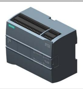
SIMATIC S7-1200, CPU 1215C, COMPACT CPU, DC/DC/DC, 2 PROFINET PORT, ONBOARD I/O: 14 DI 24V DC; 10 DO 24V DC 0.5A 2 AI 0-10V DC, 2 AO 0-20MA DC, POWER SUPPLY: DC 20.4 -28.8 V DC, PROGRAM/DATA MEMORY: 100 KB
