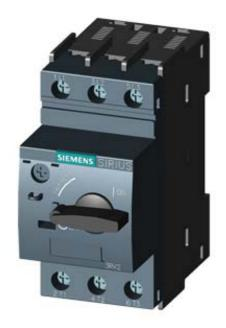
CIRCUIT-BREAKER SZ S00, FOR MOTOR PROTECTION, CLASS 10, A-RELEASE 4.5...6.3A, N-RELEASE 82A SCREW CONNECTION, STANDARD SW. CAPACITY
