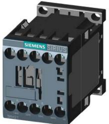
CONTACTOR RELAY, 2NO+2NC, AC 230V, 50/60 HZ, SIZE S00, SCREW TERMINAL
