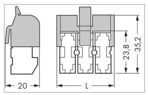
Printview: Female connector for reverse mounting; with standard marking; 3-pole; for screw or screwless mounting; with coding mask - Item No.: 272-403/272-486
