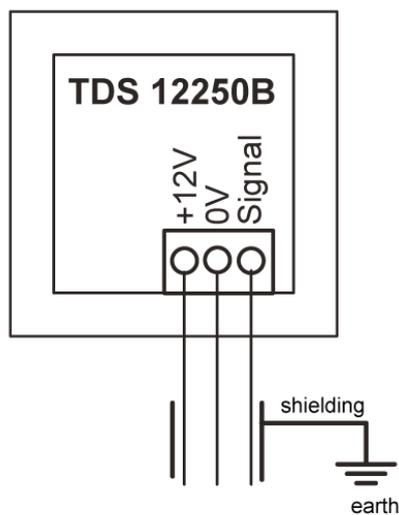
Shielded cable, to be connected to earth at the central unit or at the analog input interface (AUTOBUS shielding).
