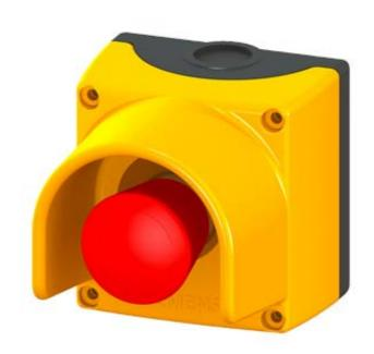
ENCLOSURE FOR 22MM PROGRAM PLASTIC VERSION 1 COMMAND POSITION YELLOW TOP PART WITH PROTECTIVE COLLAR A=EMER.-STOP40MM ROT.-TO-UNLAT. 1NC
