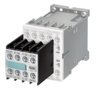
AUXILIARY SWITCH BLOCK, 22, 2NO+2NC, DIN EN50005, SCREW CONNECTION, F. CONTACTOR RELAYS A. CONTACT. FOR SWITCHING MOTORS, SIZE S00
