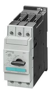
CIRCUIT-BREAKER SIZE S2. FOR MOTOR PROTECTION, CLASS 10, A-REL. 40...50A, N-REL. 650A, SCREW TERMINAL, STANDARD SWITCHING CAPACITY
