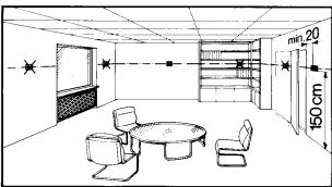
The thermostat can be fitted to most commercially available recessed conduit boxes or directly on the wall.
