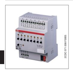
The 8-fold Binary Input BE/S 8.20.1 with manual operation is a rail mounted device for insertion in the distribution board. The device is suitable for reading out of floating contacts. The pulsed polling voltage is generated internally.
