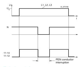
Timing interval of 5TT3 408 under/overvoltage relays
