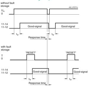
$t_{v}$ : adjustable automatic reclosing delay 0.2 to 20 s
