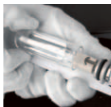
3 pull off the bulb from the drylight system
