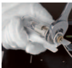
2 release the tension between the gasket and the bulb
